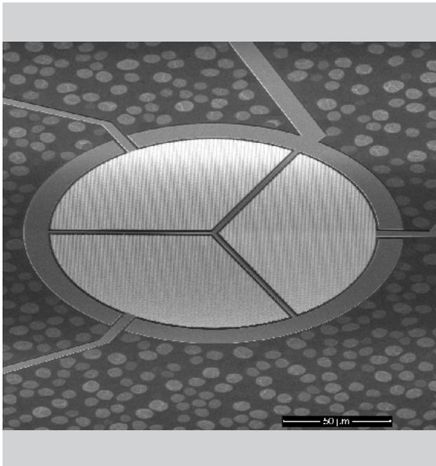
*A three-channel plasmonic pixel enables the detection of multiple wavelengths of light. Picture: Evgeniy Panchenko*
