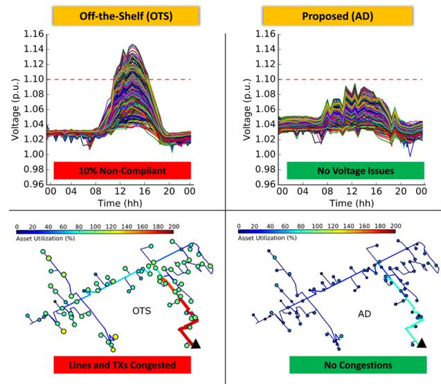
Comparison of voltage performance and network congestion between commercially available (OTS) and proposed battery energy storage controller (AD). Picture: Andreas Procopiou
