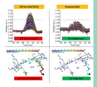
Comparison of voltage performance and network congestion between commercially available (OTS) and proposed battery energy storage controller (AD). Picture: Andreas Procopiou
