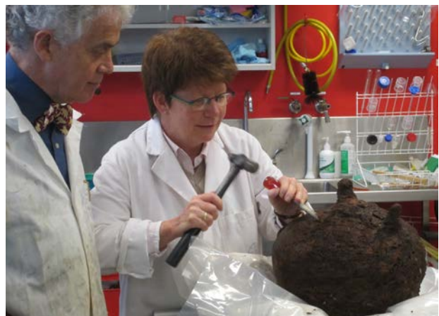
Dr Ian MacLeod (Western Australian Museum) and Marcelle Scott (Centre for Cultural Materials Conservation) deconcreting iron corrosion products prior to further analysis and conservation at Heritage Victoria conservation labs. Credit: J. Walton.
