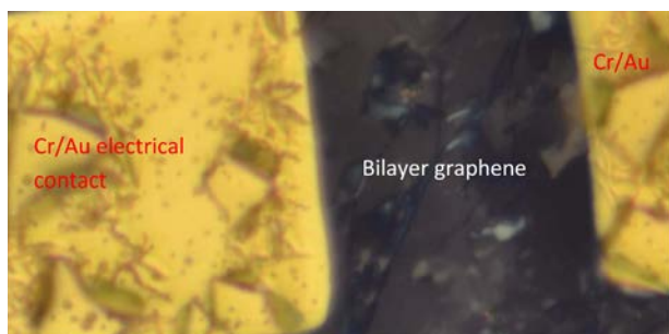
A bilayer graphene back-gated transistor with source and drain electrical contact to facilitate electrical measurement and transport. Credit: K. K. Lee.
