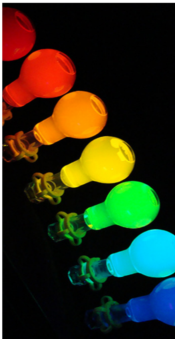
Quantum dots based on Cadmium Selenide. The luminescence varies from blue to deep red for nanocrystals varying in size from 2 to 6 nm. Credit: TL NGuyen.
